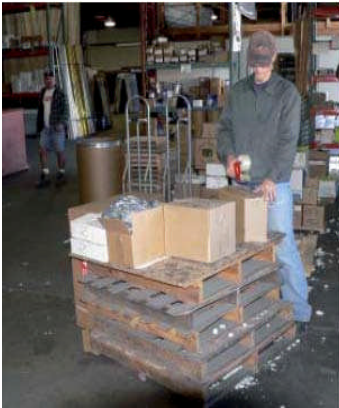
Stack pallets to create a higher work surface
