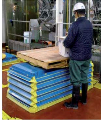
Use electric or pneumatic scissors lift
